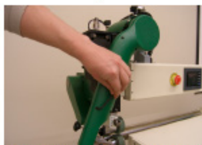
3. Loosen and remove the housing cover.
