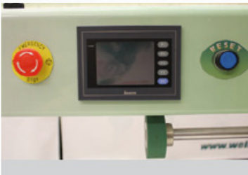
Control Panel, Reset, Emergency Stop
