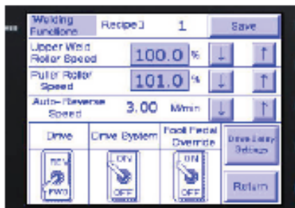
(fig.03) Welding Functions
