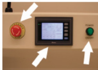
Control Panel, Power on-off, Emergency Stop
