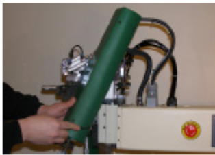
1. Loosen the protective cover...
