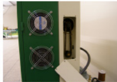
3. Remove the cover on the end cabinet...
